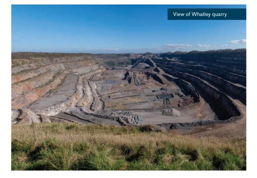
explosive charge, as well as blasting geometry and pattern – will also influence vibration levels. By adapting blast design on the south face, we are working to reduce vibration levels and thereby the way in which a blast is experienced."
